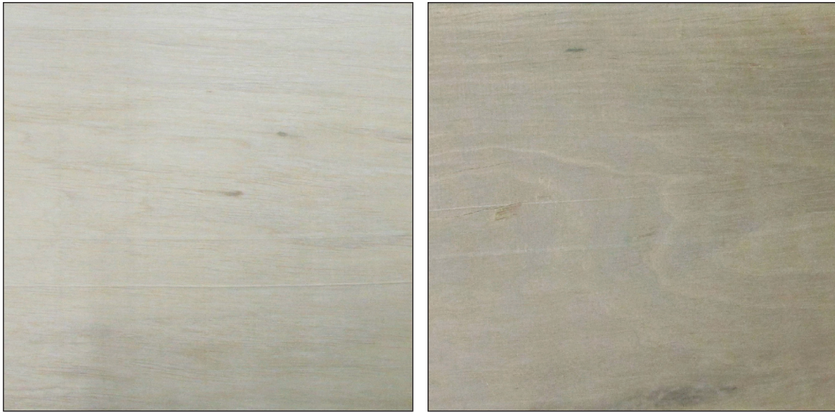
Fig. 5. Colour change as a result of acetylation on hornbeam wood (left untreated; right treated) (Fodor, 2015).
