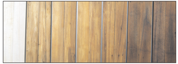
Fig. 2. Colour change of poplar wood due to different heat treatment schedules in linseed oil (Németh et al., 2012b).
